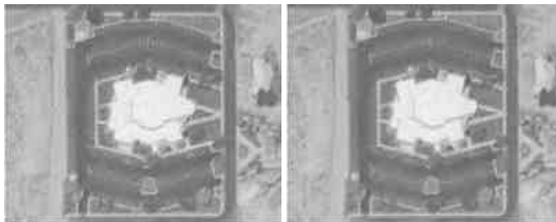
Figure 1. 12 micron scan (left) and 25 micron scan (right) on 1:24000 photography.
